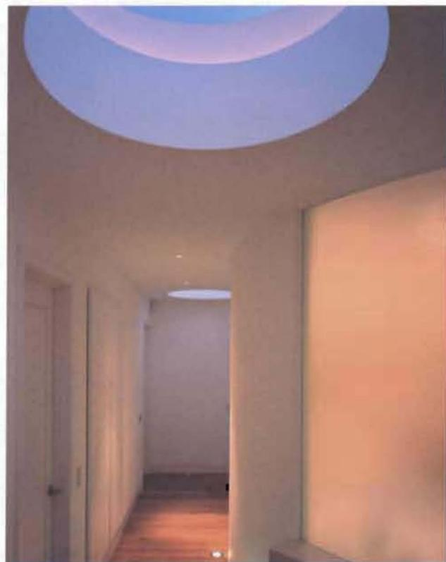
**Corridor curves:** hidden lighting in the corridor skylight and flush recessed uplights illuminate the curved wall
